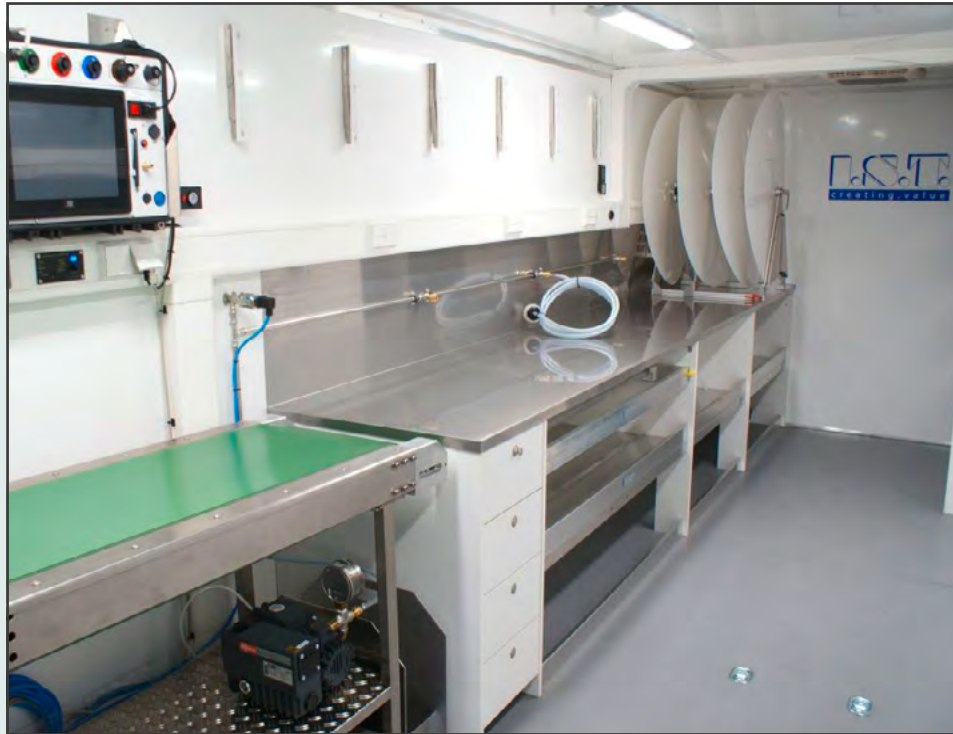
Calibration / impregnation system with documentation
