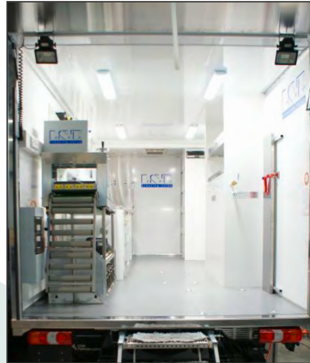
Liner calibration unit
