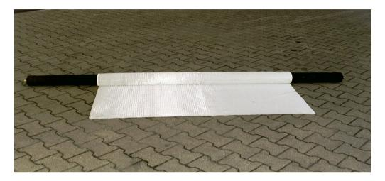
On the outside, the stranded fibre layer is now visible, it is important for a good connection to the old pipe. At the same time, the other stranded fibre layer faces the packer. This is important for a smooth impression and good resistance to HD flushing.
